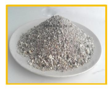
**Granulated blast-furnace slag** (**GBFS**) is obtained by quenching molten iron slag (a byproduct of iron and steel-making) from a blast furnace in water or steam, to produce a glassy, granular product that is then dried and ground into a fine powder. It is suitable for applications in marine environment, mass concreting and sulphate environment, water retaining structures, basement and other structures which require low heat of hydration.
